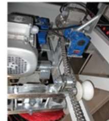
Vertical brushes are made with a chain and wheel movement on the channel.
