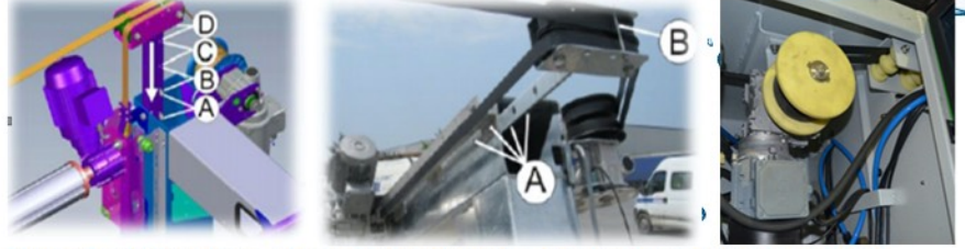
The horizontal brush up - down movement system, electric motor and is controlled by special belts.
