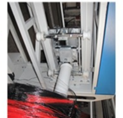
Vertical brushes are made with a chain and wheel movement on the channel.
